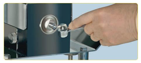
Using a 17mm or 11/16" spanner, remove the two bolts on the table clamps insert the two bolts through the two holes in the bone mill base plate.
