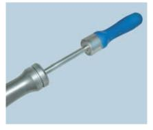
Finally, screw the Sliding Hammer Handle onto the Sliding Hammer Shaft and proceed with the extraction using short, sharp strokes.
