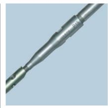
Clear any soft tissue and debris from the internal threads of the IM Nail to be removed.
