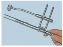
6 Connect the drill guide (CES-TD-03) to the long arms of the parallel slider bar (CES-TD-04) and secure loosely with the wing nuts.
