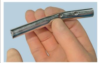
On removal of the IM nail check the external diameter at the broken end.
