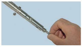
The tubular coring devices are assembled correctly and all screws are tightened
