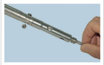
4 Attach the Jacobs cutter tube body (CES-CD-07), with two screws (CES-CD-08), onto the tubular cutter and then on to a slow speed high torque power source.
