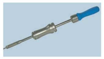
15 In the event of an unsuccessful extraction, it is possible with \*extreme caution to use the sliding hammer. First remove the offset 'T' handle from the extractor and replace it with the sliding hammer shaft (CES-SH-06) attach the sliding hammer weight (CES-SH-02) to the shaft and finally the sliding hammer handle (CES-SH-03) to the shaft.
