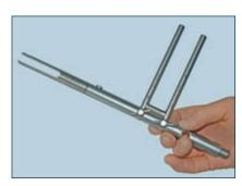
5 Connect the short arms of the parallel slider bar (CES-TD-06) to the target device main shaft and secure with wing nuts.
